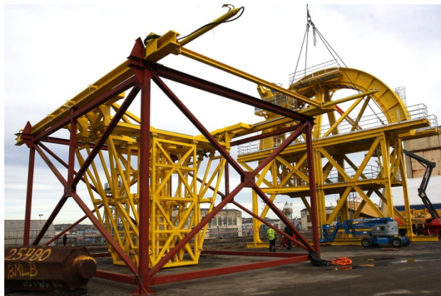
Flexible Pipe laying equipment
